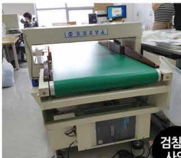
Needle & Ferrous Metal Detector
